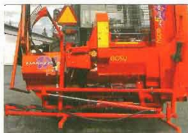
The hydraulic log lifter folds behind the machine for transport.
