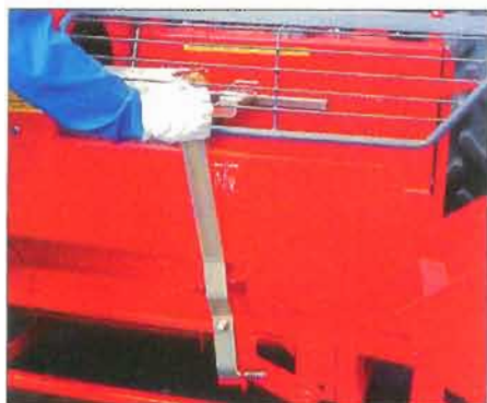
Blade height adjustment is quick and easy.
