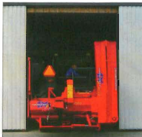
With the conveyors folded the machine is compact for transport and storage.
