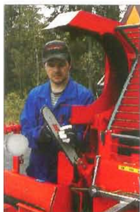
The sawbar cover is opened using a spanner. This allows easy access for maintenance.
