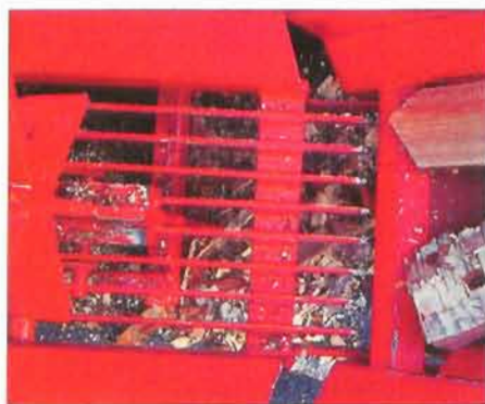
After splitting the firewood passes over a grid through which wood waste and splinters can fall.
