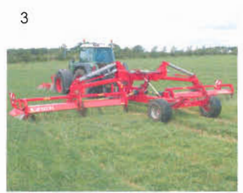
3 JF-STOLL has developed the first trailed triple-mower combination, which has a working width of 12 m.
