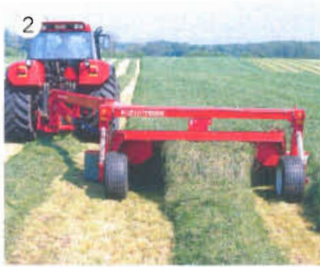
2 JF-STOLL mowers have a working width from 1.7 m and up to 12 m. They can wide spread and make single or double swaths.
