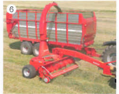
6 The JF-STOLL Precision Chop Forage Harvesters are available with 1.6-3.1 m pick-up as well as direct-cut headers and maize headers
