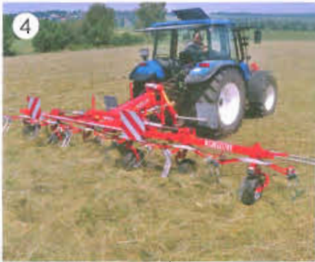
4 JF-STOLL manufactures rotary tedders from 4.5 to 9 m working width.
