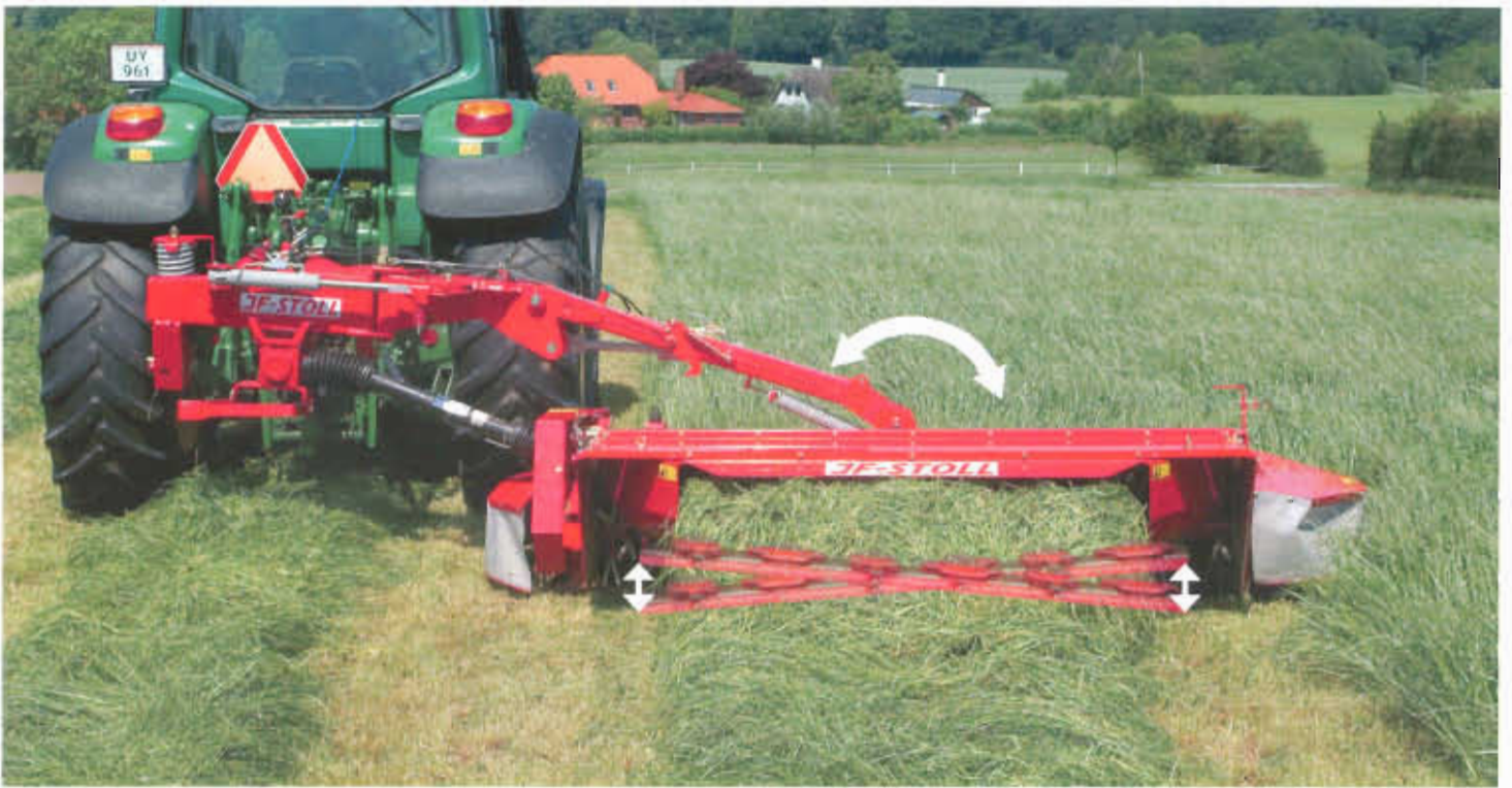
The GX-machines have center suspension which ensures good ground adaptation.
