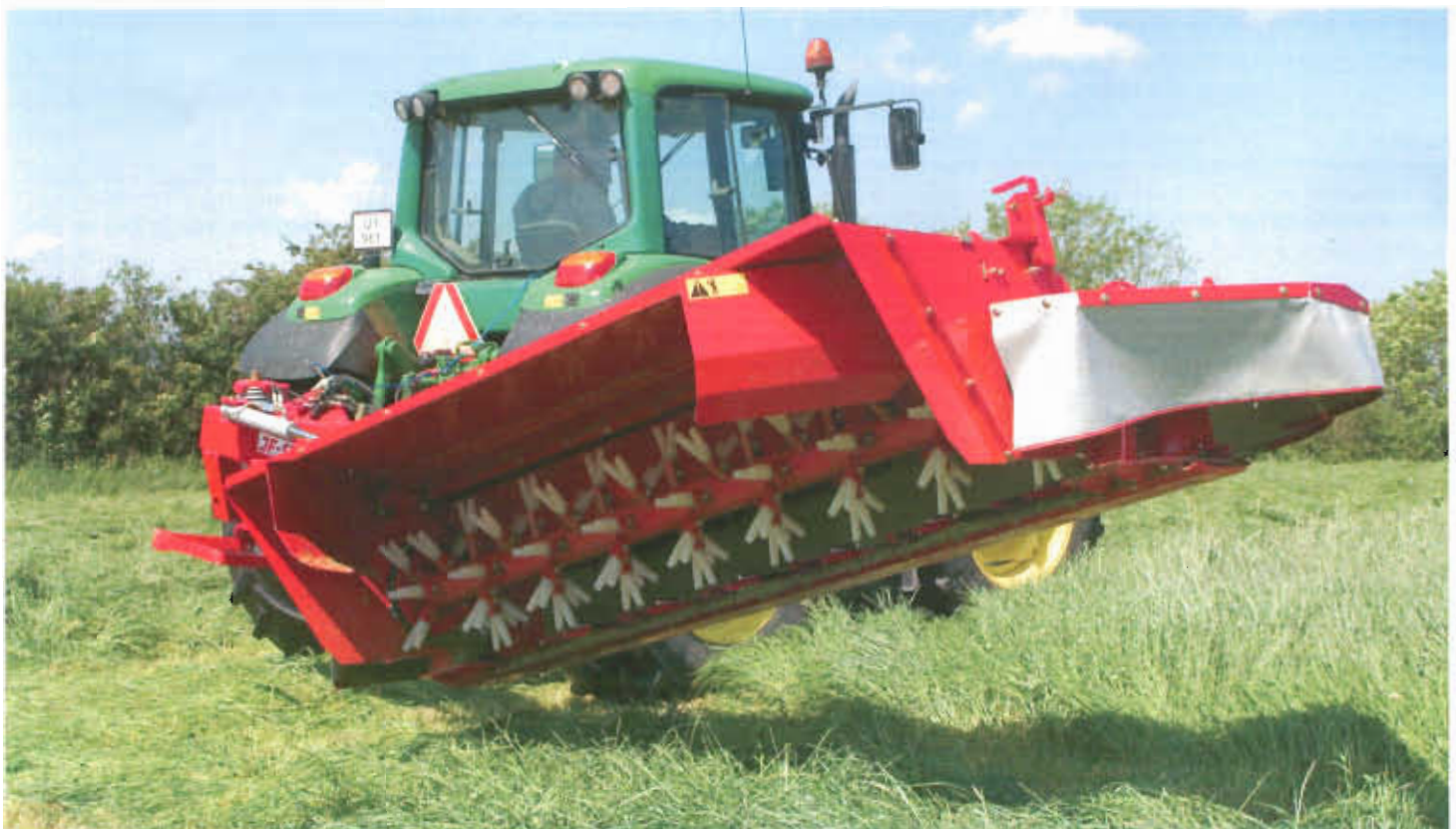
The GX-SM models are equipped with JF-STOLL's strong and effective PE finger conditioners.
