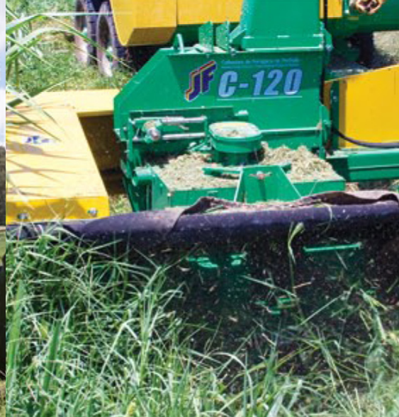
JF C120 with JF 1300 Grass Head* Harvests green grass / picks up wilted grass / 1,30m working width
