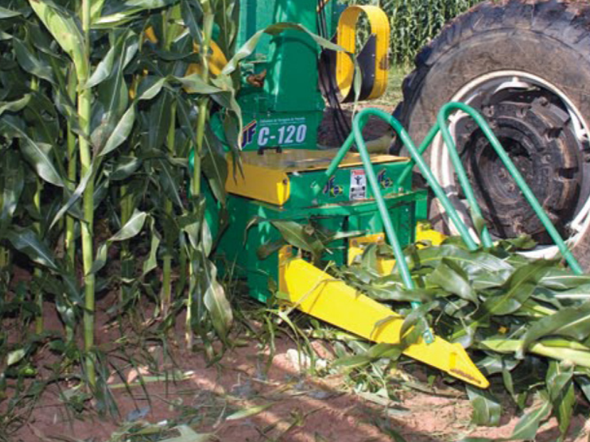
JF C120 with JF 500-4 two row head* Harvests 2 rows of maize or sorghum with distance between rows of 45 to 55cm
