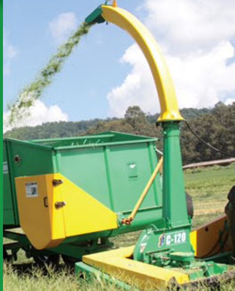
JF C120 with JF 1300 Grass Head* Harvests green grass / picks up wilted grass / 1,30m working width
