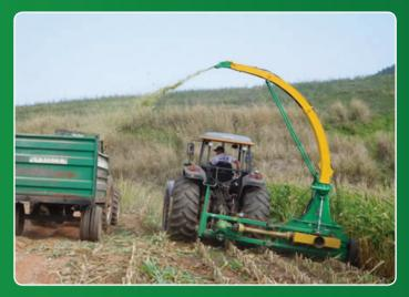
New gathering platform with higher intake capacity, Longer durability of gears, Less stress for tractor
