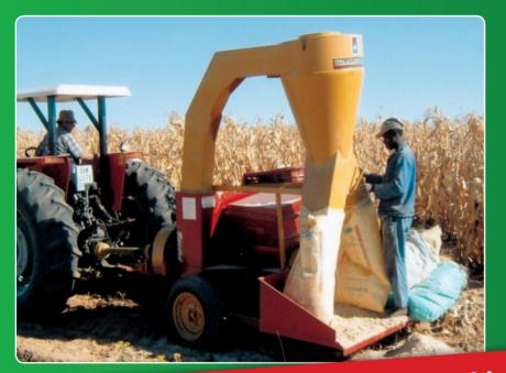
An additional beater easily handles material with a high moisture content and makes sure that material is presented correctly to the feeding tray, and by means of the auger it is fed evenly through to the rotor housing.
