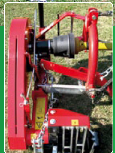
Compact 3 point hitch designed for small tractors.
