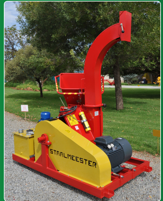
HJ-4 Chipper modified to run with an electrical motor.
