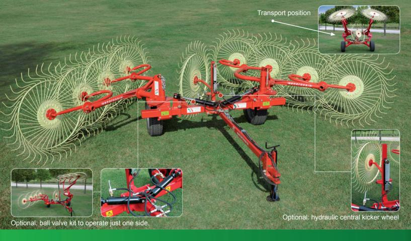
Enoagricola Rossi offers the top of the line in affordable 8, 10 and 12 wheel rake carts. Its simple compact design keeps moving parts down to a minimum, eliminating excessive wear points. A newly designed transport caddy gives a high ground clearance of over 20", which keeps the transport bar away from cut hay when raking under heavy conditions.
