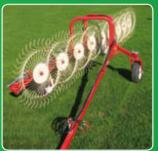
Enorossi pull type rakes (RT7-RT9) are equipped with three wheels (or four for the RT 13) to ensure greater stability during raking and transport. They are used for raking hay and all types of forage. All forage is gathered in a soft windrow without destroying the leaves, maintaining a high nutritive value. They are extremely suitable for gathering on small allotments with uneven windrows. Tooth  $\varnothing$  6.9.
